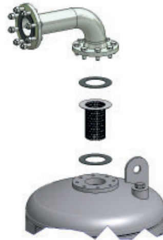
Disassembling of desiccant sieve
